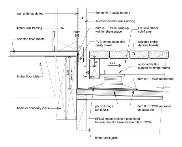
duroTPO-T30 - timber raft floating deck-wall detail - type 2
